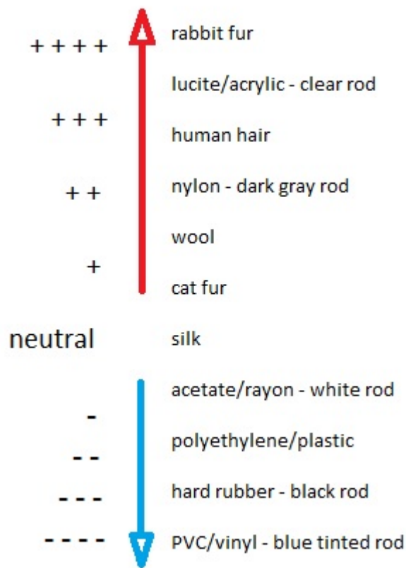
Figure 2: A relative electronegativity ranking for some common materials. Here “+” is electron donating, “-” is electron accepting. The further apart the materials, the greater the charge transferred, resulting in greater static charge.
