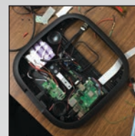
Prototype 6 This was the "looks-like, works-like" device that went to the Consumer Electronics Show. It was hand-soldered and featured a redesign of the voice-interaction model.
