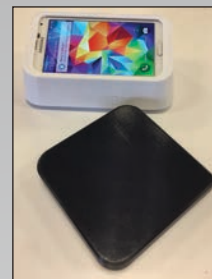
Prototype 3 Able to take scale sensor data and weight values, this device sent the information to the internet. A phone was placed in a plastic housing that served as the display or hub for the scale. The weight of an object placed on the black box would be sent over the internet and appear on the hub.
