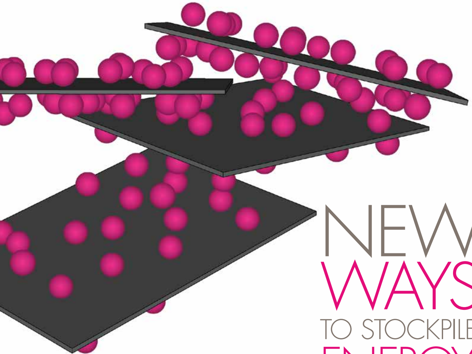
This schematic is of a 3-D supercapacitor utilizing graphene sheets studded with nano-oxide islands.
